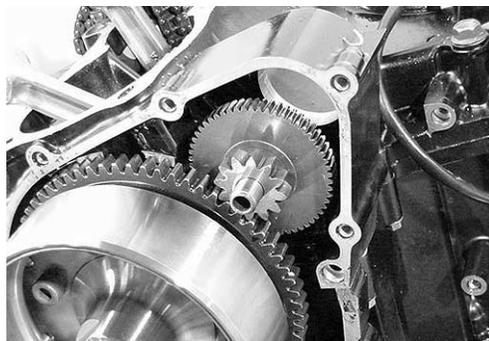
**GENERATOR ROTOR/STARTER CLUTCH**
