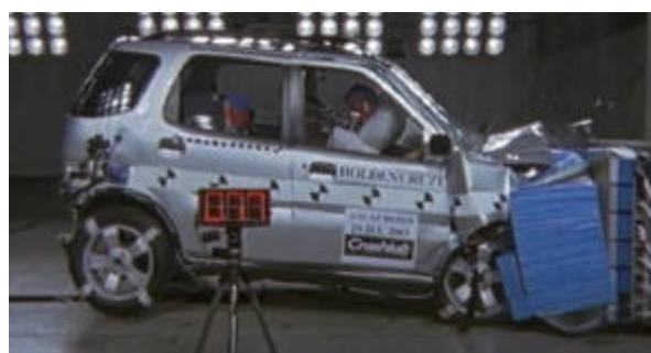
Offset crash test at 64km/h
