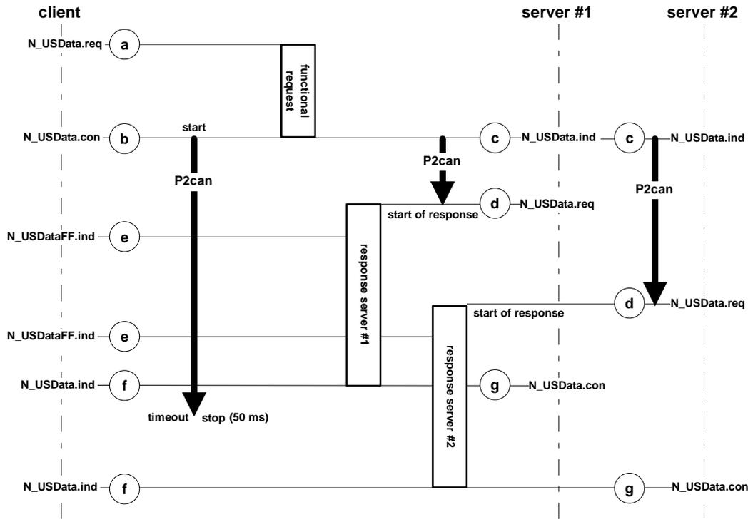
**Figure 2 — Functional OBD communication: Default response timing**
