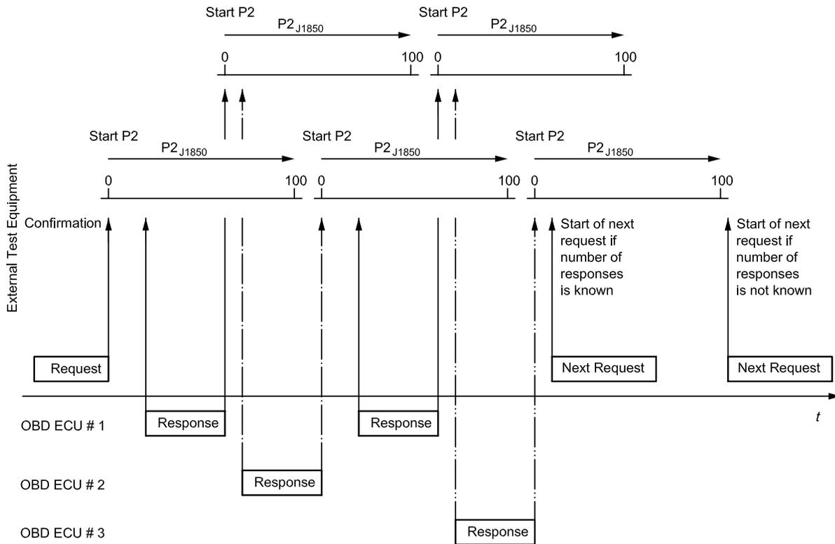
Figure 5 — SAE J1850 application timing parameter overview
