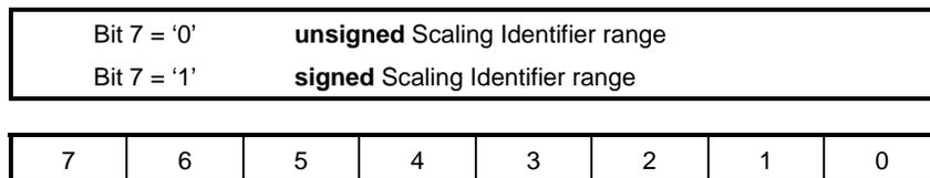
Figure E.1 — Unsigned/Signed Scaling Identifier range encoding
