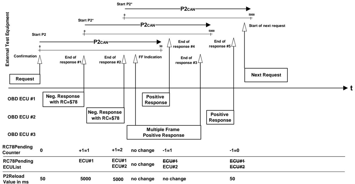
Figure 13 — ISO 15765-4 — Negative response code RC=\$78 handling overview
