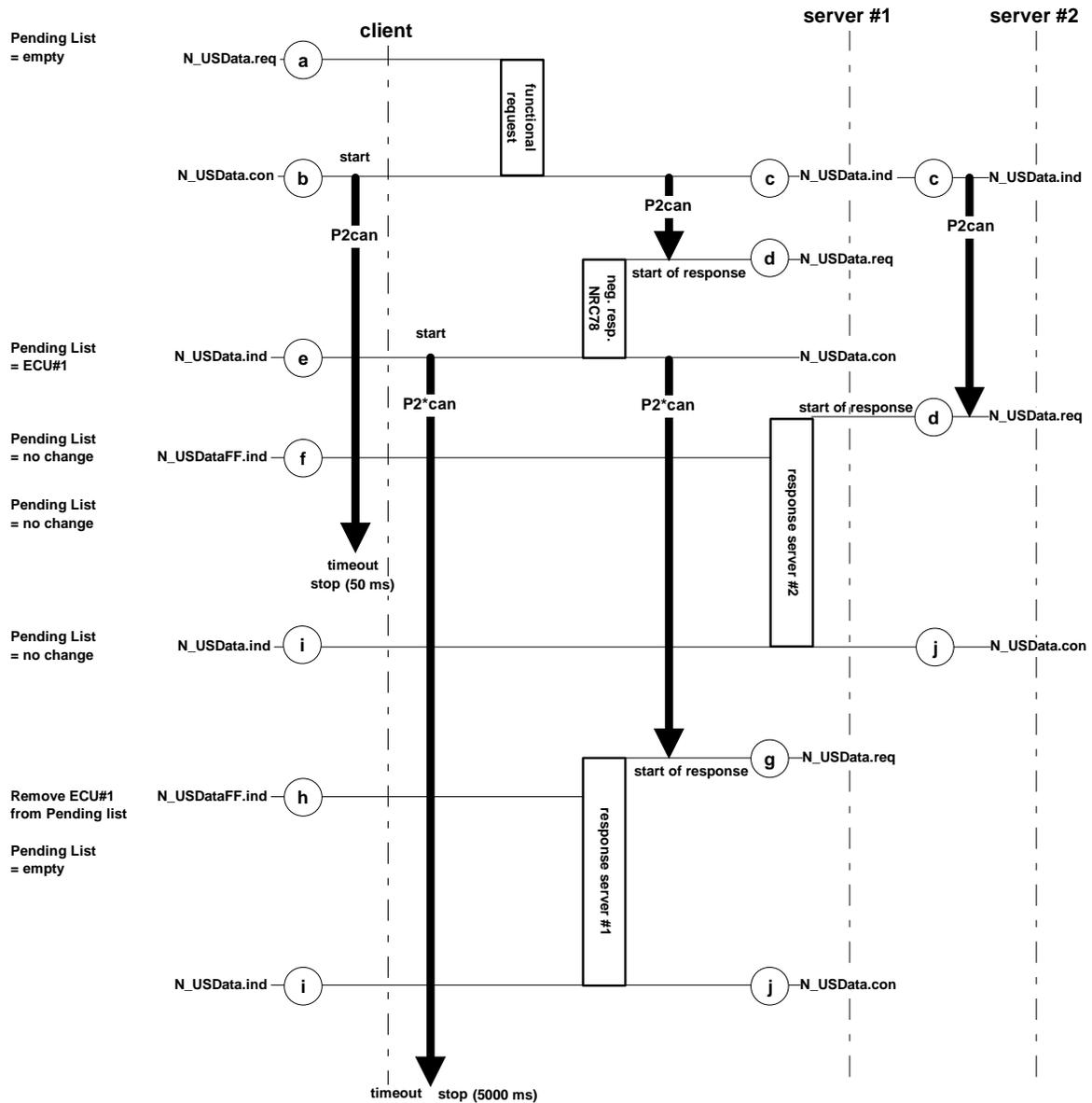
**Figure 3 — Functional OBD communication – enhanced response timing**
