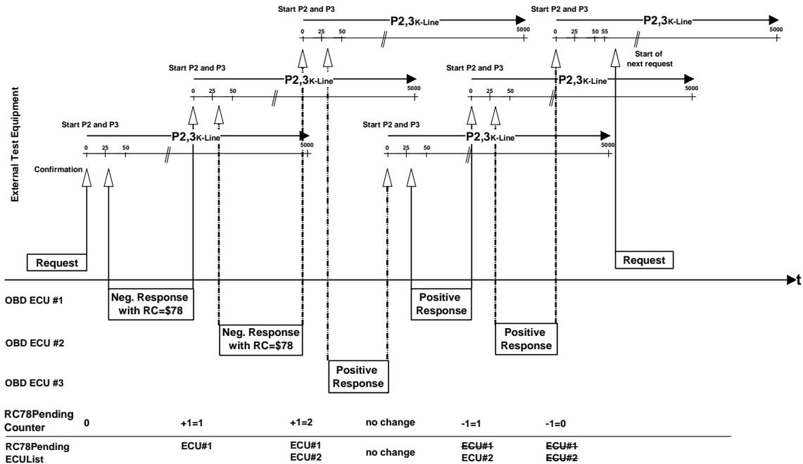
Figure 11 — ISO 14230-4 — Negative response code RC=\$78 handling overview
