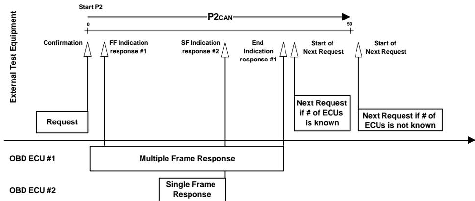
**Figure 8 — ISO 15765-4 application timing parameter (Single and Multiple Frame Response Messages within P2<sub>CAN</sub>) overview**
